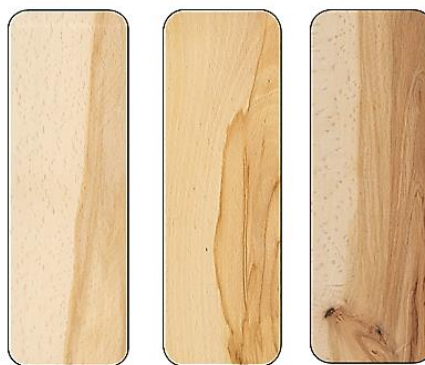
Fig. 1 The colour of the false heartwood beech (on the samples on the right) and mature wood (in the samples on the left).
